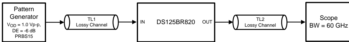
Figure 10. Test Setup Connections Diagram
